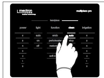
To start the CLEAN function while the screen flashes press the foot pedal once and release it; the screen stops flashing and the irrigation circuit begins to be filled up;
