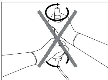
**! WARNING:** Do not attempt to unscrew or turn the connector when disconnecting the handpiece. The connector could get damaged.
